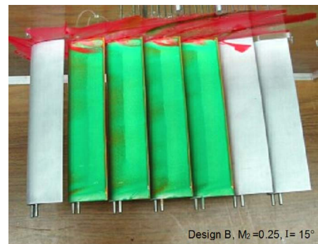
Fig. 9 Flow uniformity and periodicity confirmed by blade surface flow visualization (S.S.)
