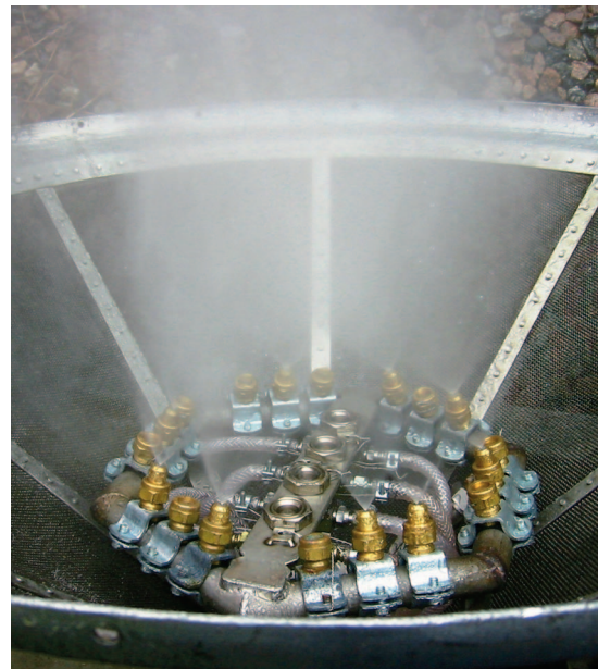
Fig. 3 Water wash manifold with eight nozzles giving 75 \mu\text{m}_{\text{VMD}} droplets at 4.3 l/min
