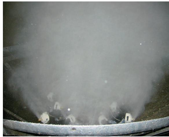
Fig. 2 Water wash manifold with 12 nozzles giving 25 \mu\text{m}_{\text{VMD}} droplets at 4.4 l/min
